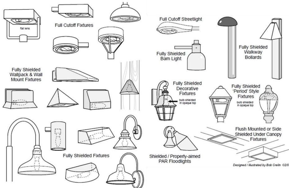
*Examples of a range of cutoff shield styles.*
