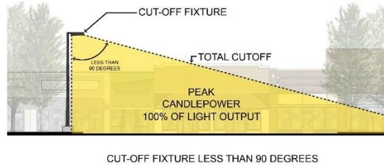
*Examples of lighting fixtures without cut-offs or shields, and those designed with a cut-off to present light spill onto adjacent property.*
